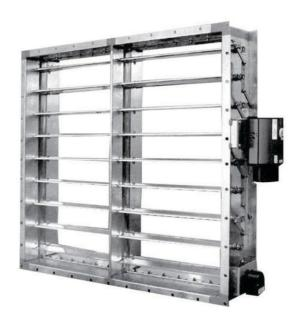
Tunnel Damper shown with internally-mounted actuator protected by a thermal enclosure. Includes factory supplied and mounted terminal box, conduit, and blade-mounted proximity switch.
